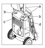
The standard accessories (spray gun and spray lance (a), nozzles (b) foam sprayer (c)) can be stored on the pressure washer.
